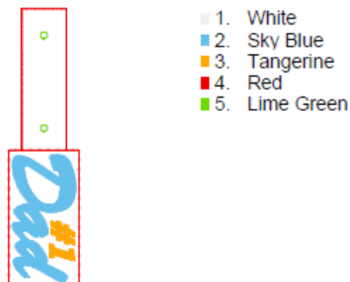
No1dad Snaptab Final.pes 25.60x99.40 mm; 2,378 stitches 5 thread changes; 5 colors
