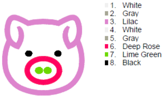
Fig 4x4 (3 Inch).pes 75.40x74.30 mm; 3,788 stitches 8 thread changes; 6 colors
